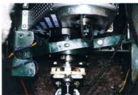
'Clever box of tricks' (top): Morse-type lever (right) operates clutch for using diesel just for charging
