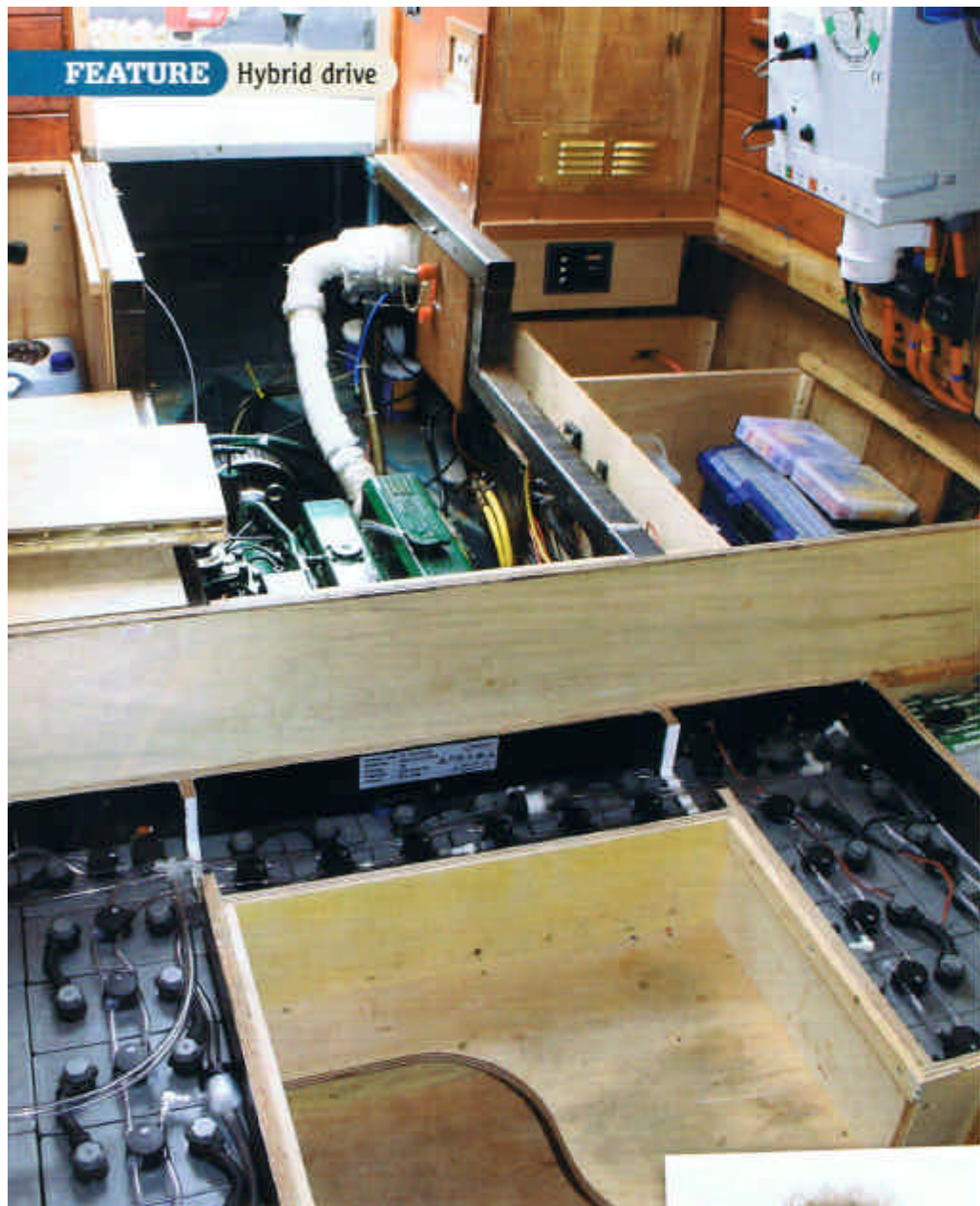
Twenty-four two-volt batteries should last ten years if charging is properly managed
