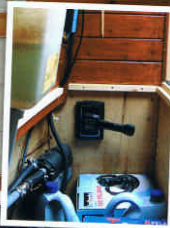
'Clever box of tricks' (top): Morse-type lever (right) operates clutch for using diesel just for charging
