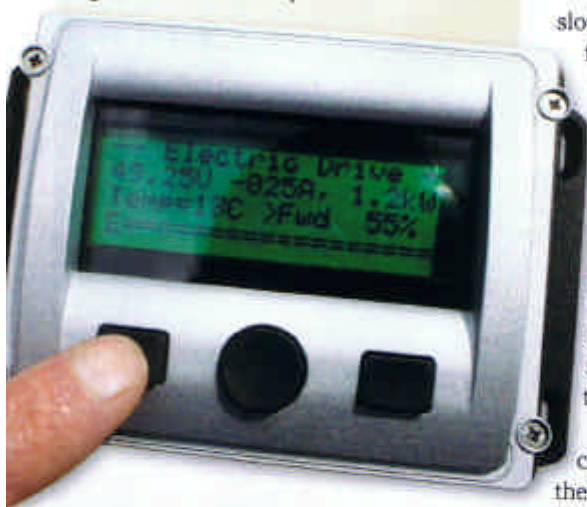
Control box with buttons for Slower (left), Stop (centre) and Faster, plus info readout
