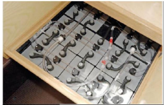
Twenty four cells are used to provide the Hybrid power supply of 48V. Two battery bank sizes are available, 400Ah giving 4 to 5 hours of electric drive and 800Ah providing up to two days of electric drive. A combined watering and venting system is provided to allow top up from one central point and simple safe venting of gases overboard.
