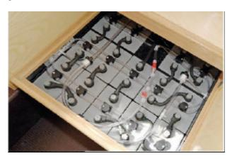
Twenty four cells are used to provide the Hybrid power supply of 48V. Two battery bank sizes are available, 400Ah giving 4 to 5 hours of electric drive and 800Ah providing up to two days of electric drive. A combined watering and venting system is provided to allow top up from one central point and simple safe venting of gases overboard.
